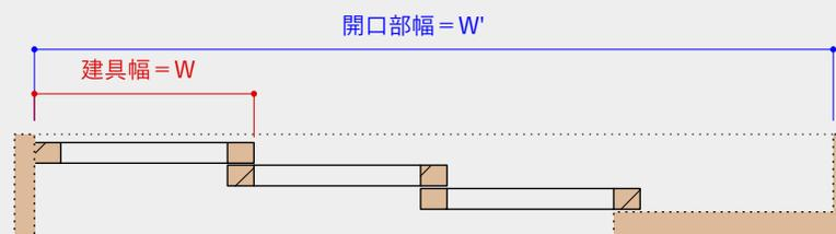
$$\text{建具幅} : W = \frac{\text{開口部幅} W' + \text{框幅} : 50 \times 2}{4}$$
